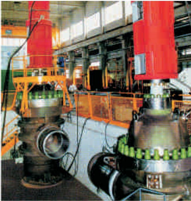
G12 Gate Valve 42 inch ASME Class 1500 with hydraulic linear actuators
