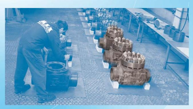
A 44 swing check valves with pressure seal bonnet
