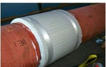
Pipe Body Failure @ 4,260 psi
