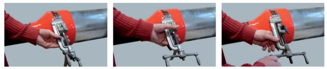
**2.** Introduce the strap laterally in the clamping tool, push the clamping tool up to the loop, press the holding lever and tighten the strap by turning the crank.
