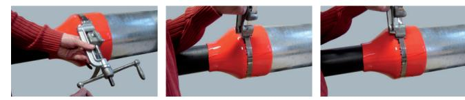
3. When reaching maximum stress, slowly bend over the strap about half a turn while releasing the crank.
