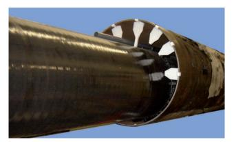
Fix plastic support with included clip at the inner wall of the casing pipe. Cut into suitable length if necessary. Space has to chosen suitable according to the cavity in the support segments.
