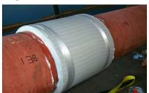
Pipe Body Failure @ 4,260 psi
